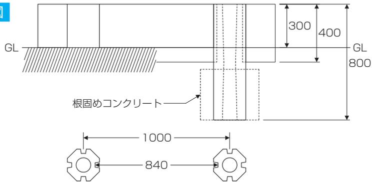
柱と柵板の隙間は片側7.5mm
